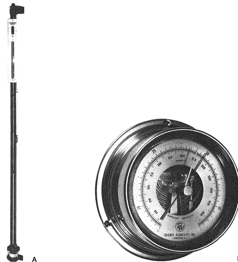
Figure 4.2 Pressure-measuring instruments. (A) Mercury barometer, in which the atmospheric pressure is balanced by the mercury in an evacuated tube. The length of the mercury in the tube is a measure of the pressure; consequently, pressure is frequently expressed in terms of length. Thus, standard atmospheric pressure (1013.25 mb) is 760 mm of mercury. (B) Aneroid barometer, in which the atmospheric pressure compresses a partially evacuated flexible metal box. The changes in the size of the box with pressure are converted by a mechanical linkage to the position of the pointer on the dial. In the example shown, the scale indicates the pressure in millibars (inner scale) and inches of mercury (outer scale). [Courtesy of Science Associates, Inc., Princeton, New Jersey.]
