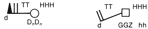
Figure 13.9 Model for plotting rawinsonde observations and reports from aircraft on upper-air charts.
