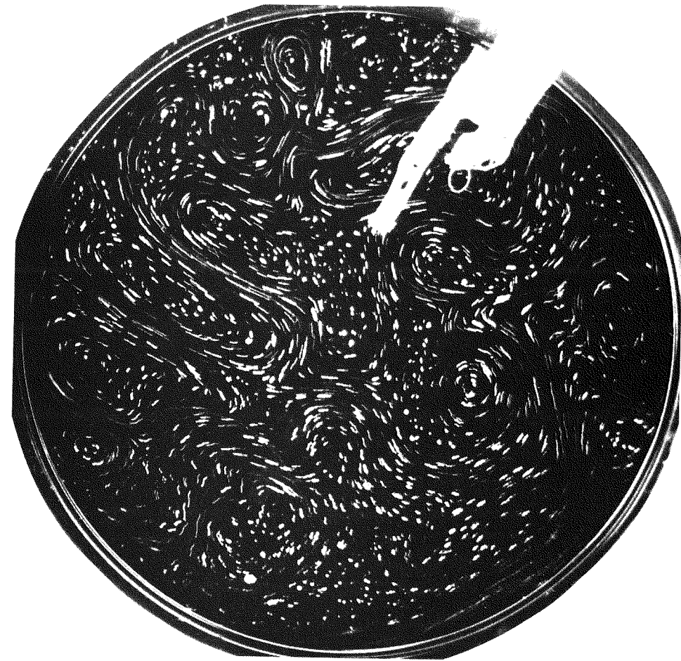
Figure 9.13 Photograph of flow pattern in "dishpan" laboratory model of the general circulation. [Courtesy of D. Fultz, University of Chicago Hydrodynamics Laboratory.]
